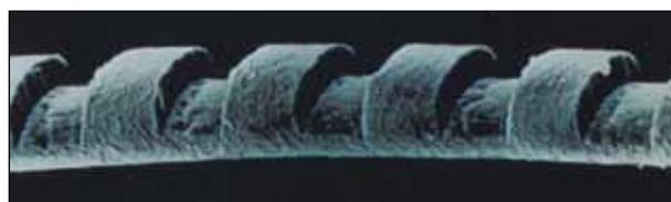
**Figure 6.** Excimer laser etchings in a human hair, demonstrating precision without thermal damage.
