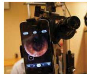
Figure 3. A SteadyPix Telescope Photo Adapter attached to a slit lamp.
